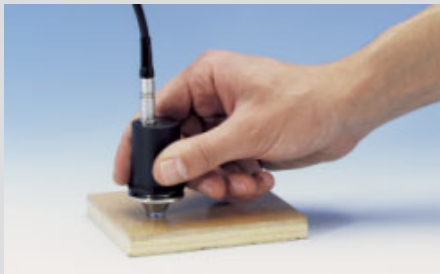
Thickness measurement of a double-layer coating applied on wood
